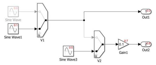
In R2016b, the code generator produced this code in the VariantMergeReuse step function: #if V == 1 || V == 2
