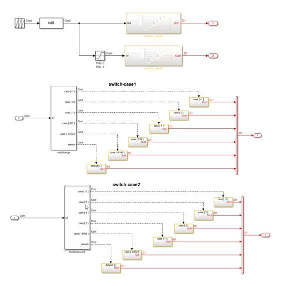
In R2018b, the code generator produced this code for the outofrange and twoCasesLeft Switch Case blocks.
