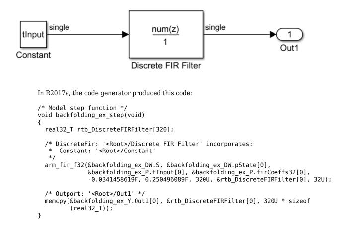
The generated code contained the temporary variable rtb\_DiscreteFIRFilter and a memcpy function for copying data from rtb\_DiscreteFIRFilter to the destination variable backfolding\_ex\_Y.Out1.
