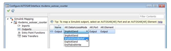
When you generate code, in rtwdemo\_autosar\_counter.c, the model step function uses Rte\_IWriteRef to write the sender port data.
