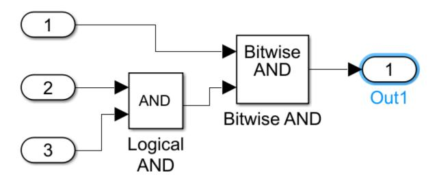
To generate code, in the Configuration Parameters dialog box, set the **Operator to represent Bitwise and Logical Operator blocks** parameter. Choose from these settings:
