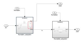
Beginning in R2014b, AUTOSAR code generation supports branching outside the runnable. This modeling pattern can potentially generate more efficient C code, for example, with fewer global variables and fewer block I/O buffers.
