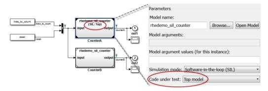
If you set the Model block parameter, **Simulation mode** (SimulationMode), to Software-inthe-loop (SIL) or Processor-in-the-loop (PIL), the software provides a new parameter **Code under test** (CodeUnderTest) with the following options:
