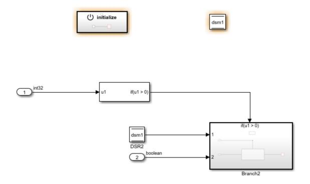
Inside the subsystem Branch2, a bus is output from the Subsystem block and written by a Data Store Write block to the Data Store Memory dsm1 in top-level model.
