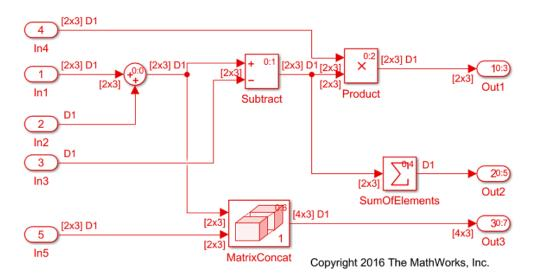
In R2017a, the code generator can reorder the block execution order so that the Matrix Concatenate block executes before the Subtract block and the Sum of Elements block executes before the Product block. Reordering block operations eliminates the two temporary arrays, the two variables, and their associated data copies from the generated code. The blocks can use the same variable for the input and output.
