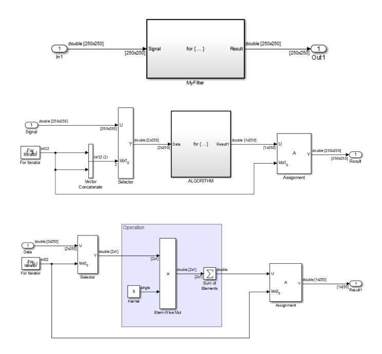
ALGORITHM, which is nested in MyFilter. Both subsystems contain a for Iterator block, a Selector block, and an Assignment block.
